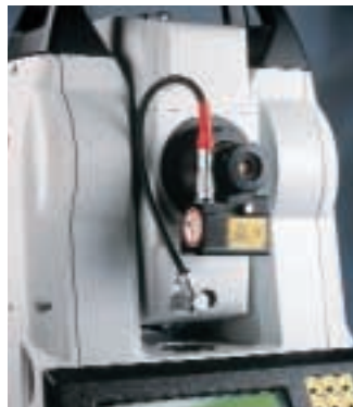
Laser pointer for setting out locations on site according to the design data
