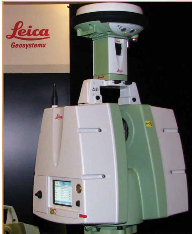
The new Leica ScanStation C10 scanner, which features onboard control plus attachments for accessories like GPS, was on display in the exhibit area.
