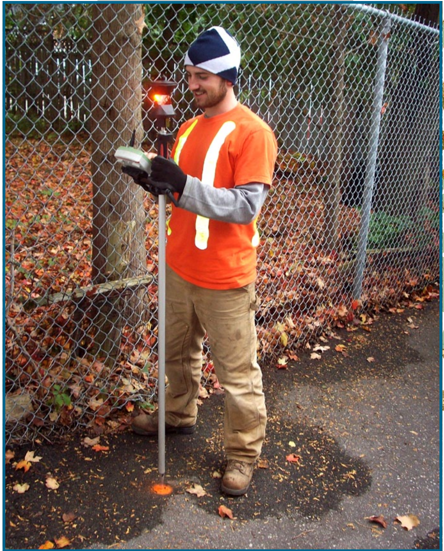
At least one Van Harten survey crew has completely abandoned traditional methods of setting control points and traversing a site, relying instead on a pole-based GPS and TPS system.
